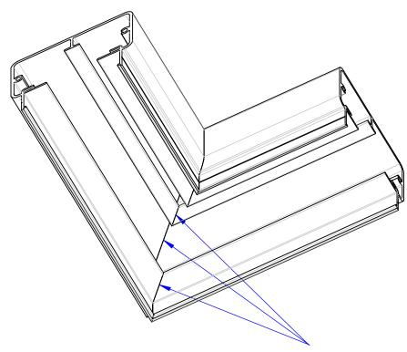
Weld underside of seams only
